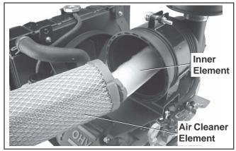
Figure 14. Air Cleaner Element and Inner Element.
